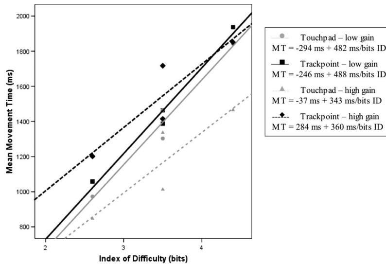
Figure 1. Mean movement times (ms) as a function of ID (bits) and gain for the touchpad and mini-joystick (Experiment 1).
